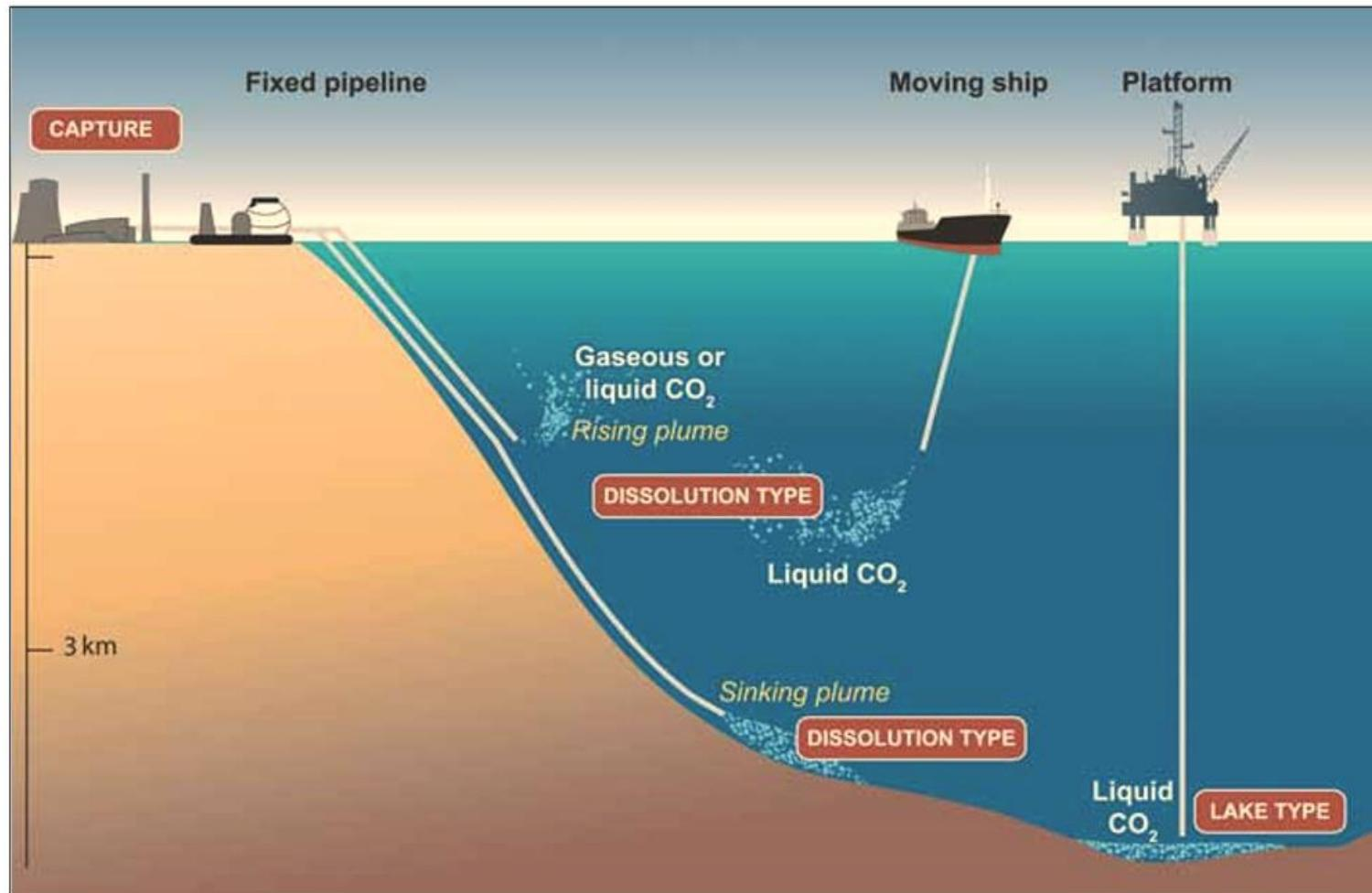
**Figure SPM.5.** Overview of ocean storage concepts. In “dissolution type” ocean storage, the CO<sub>2</sub> rapidly dissolves in the ocean water, whereas in “lake type” ocean storage, the CO<sub>2</sub> is initially a liquid on the sea floor (Courtesy CO2CRC).
